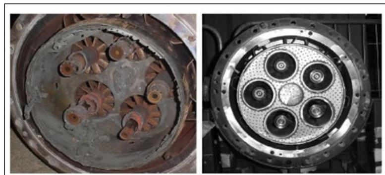
Figure 1.9: Burner assembly damaged by combustion instability (left) and new burner assembly (right) (Goy et al. [8]).
